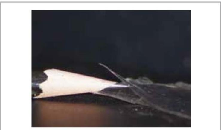
**Figure 12b.** Mica: made of sheets of silica tetrahedra. Source: Nikhil Fernandes.
